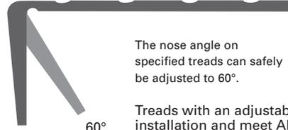
The nose angle on specified treads can safely be adjusted to 60°.
