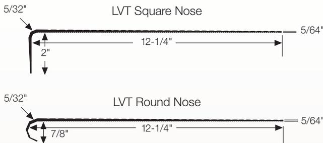
Adjustable nose portion should be secured with contact adhesive or FlexTape according to FLEXCO<sup>®</sup> instructions.
