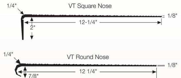
Adjustable nose portion should be secured with contact adhesive or FlexTape according to FLEXCO<sup>®</sup> instructions.
