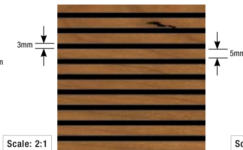
W8* Type: Channeled Groove Size: 5mm profile with 3mm groove NRC: 0.80**
